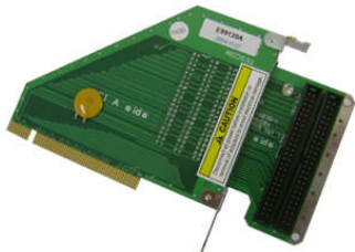
E99120A, PCI to 100pin adaptor, for the right side motherboard.
