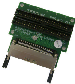
E99110D, 100pin to CardBus adaptor.
